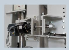
The new electrical bracing of the 2nd filling device is unique on the market. This efficient, electrical solution allows for a quick and safe connection of the machine base part with the 2nd filling device. With this, a safe and fully-automatically opening and closing of the 2nd filling device is possible. Quick and short mould change and maintenance times are therefore the major advantages.
