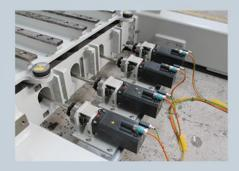
The single pallet machine ZENITH 1500 is working with an innovative servo compaction system named UltraDynamic. This high-quality vibration system is characterized by a very high compaction and extreme dynamics and therefore guarantees a quick and efficient high-quality production. Especially for large-volume components and high-quality products, which are produced with pre- and intermediate vibration, this vibration system is very profitable.
